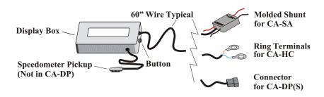
The Cycle Analyst picks up the vehicle speed information using either a spoke magnet, or in the case of the CA-DP device, through the hall sensor signals from a brushless motor controller.
